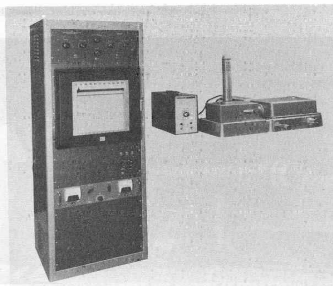
Fig. 8. Perkin-Elmer laser Raman spectrophotometer source mounted on top of instrument.
